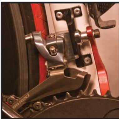
HFK 5mm spacer and 30mm bolt used to space K-Edge away from seat tube on this Cervelo R3.
