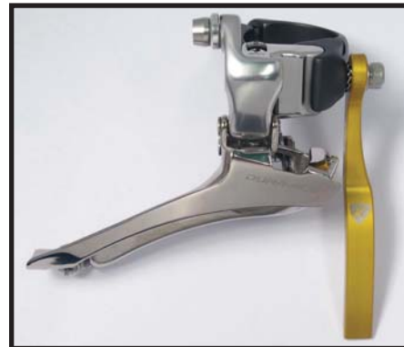
Assembly of a K-Edge and front derailleurs to a "Braze-On" clamp.
